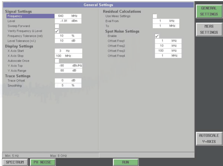
Fig. 2: Setting of global parameters for phase noise measurements: The basic measurement parameters (carrier level and frequency, display ranges, etc), the residual FM/φM measurement range, as well as discrete offset frequencies of interest are entered here.
